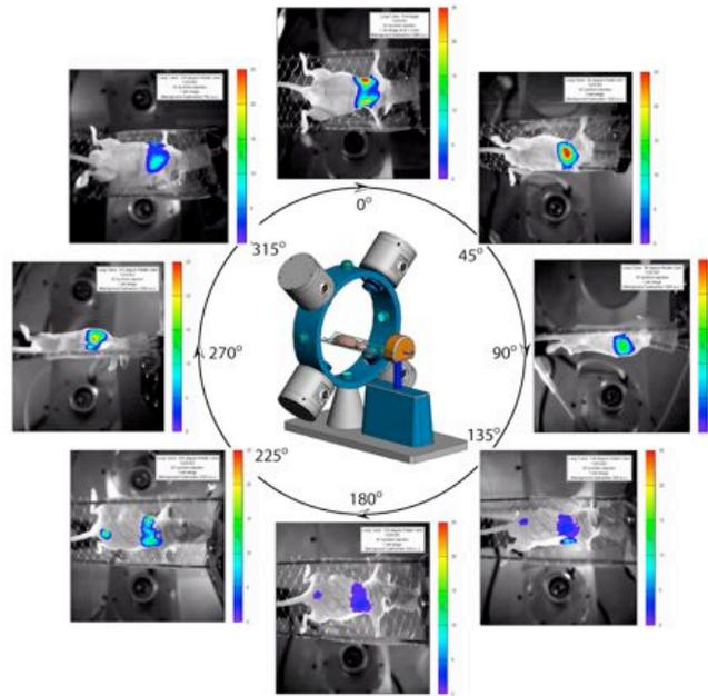
**Figure 6.1 – Schematic of Light Emission Tomogram.** A schematic diagram demonstrates the function of the LET apparatus. Images are taken from five CCD cameras representing all the angles within  $360^\circ$  and reconstructed into a 3D image.
