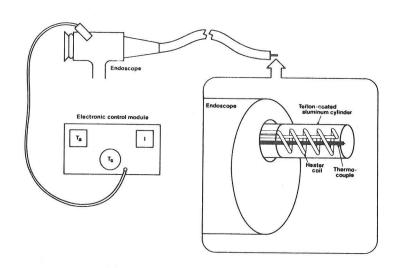
A thermocouple in the tip maintains the temperature at the level (100-180°C) set on a control panel (Figure 8A). The Seattle group first designed a 6.4 mm diameter probe and then a 3.2 mm probe which could be passed through a flexible endoscope (Figures 8B and 8C).
