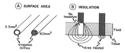
By reducing the size of the irrigation orifice, the area of the electrode face is increased (Figure 12A), reducing the energy density, and possibly reducing tissue injury. On the other hand, the use of an un-insulated electrode allows the current to dissipate through fluid to cover a larger area (Figure 12B). In this case, the energy density is too low for effective hemostasis.
