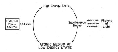
If one now places focused mirrors at each end of the tube containing the active medium, the photons released by spontaneous decay will oscillate very rapidly between them. In doing so, they greatly accelerate the decay of the active medium back to its low energy state resulting in the stimulated emission of monochromatic light.<sup>29</sup> (Figure 14)
