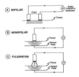
Whether a current will fulgurate is dependent on the voltage applied. Whether the current will "cut" or "coagulate" is dependent on the waveform applied. Examples are shown in Figure 10.
