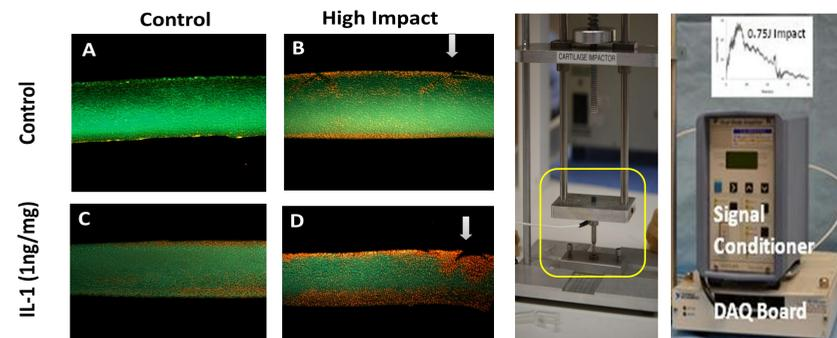
Fig 1. (A-D) Impact (white arrows) and IL-1 increased cell death (Red=dead cells, Green = live cells) in cartilage explant with impact energy of 15J/cm<sup>2</sup>. (E) A drop-tower apparatus to create impact injury.
