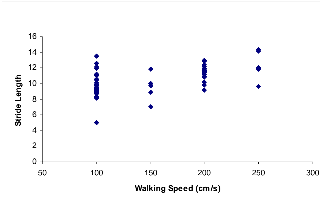
Figure 5. Stride length increases with increasing treadmill speed.
