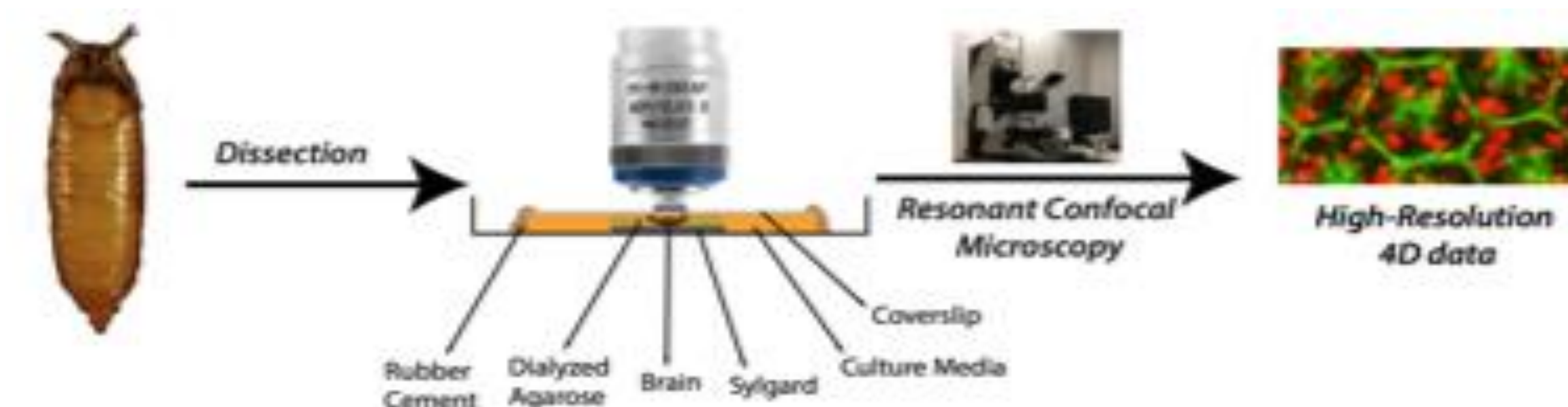
Figure 3. Schema of live imaging technique of Drosophila brains.
